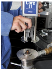
3. Slide Electric Motor to Remove
